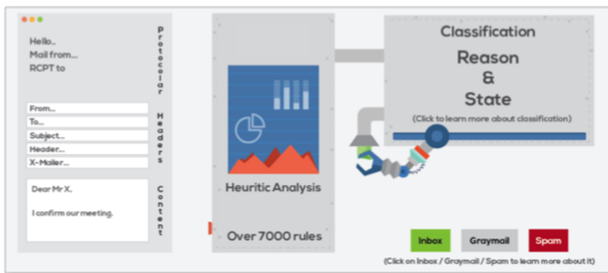
Figure 5 – the Vade Secure filtering process, using heuristic analysis to classify emails and assign messages to inbox, graymail or Spam.
